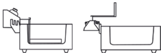
Fig. 4: Hinged position of frying head for oil removal
