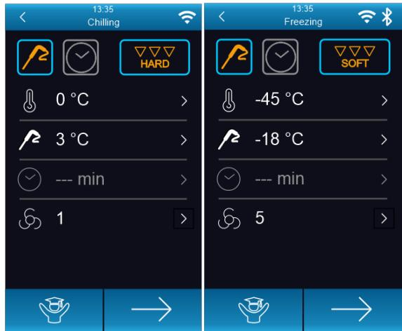
The cycle selected will use the preloaded settings for that cycle, but pressing area makes it possible to change the main settings, within the permitted range, which are shown on the display. To change all the various set points for the phases of the selected cycle, expert mode can be enabled by pressing area . Once all the settings have been done, press area to terminate the phase. The screen summarising all the setting data for the cycle will appear, as shown below.
