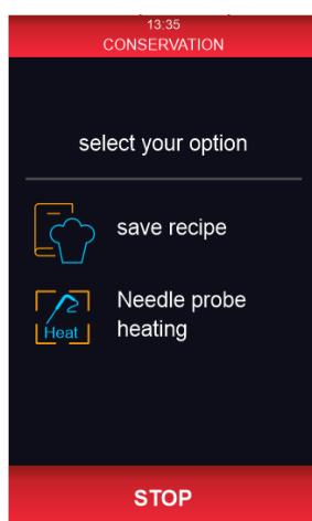
In time controlled cycles, , pressing the **STOP** key will bring up the screen granting access to the following functions.
