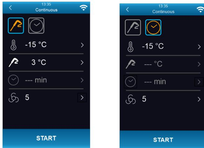
Continuous cycle-needle probe    Continuous cycle-time control
