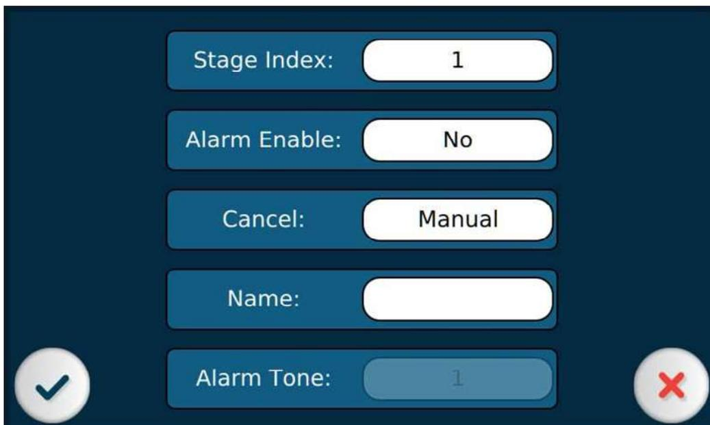
“Stage Index” can choose to set alarm for stage 1, 2, 3 (if you have more than 3 stages); Alarm Enable: click on “yes” ; click on “cancel” can select means of cancelling alarm, either manual or automatic; click on “name” to **edit name** for this alarm (**Must set!**). Manual: When alarm rings, there must be a physical action to stop alarm Automatic: After ringing for a few seconds it will automatically stop
