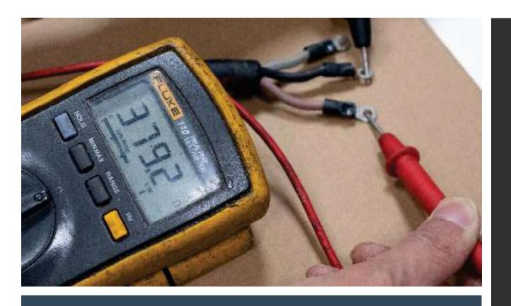
• (19048693 IE-35-D / CB-70A) Measuring L1&L2, you will get resistance of  $400\Omega + / - 10\%$  if it is under normal condition.
