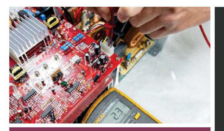
Measuring the location in the left photo and you should get very low resistance if the transformer is under normal condition.
