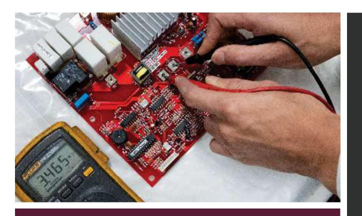
• Measuring G&E and you should get a very high resistance such as  $3.46M\Omega$  if it is under normal condition.
