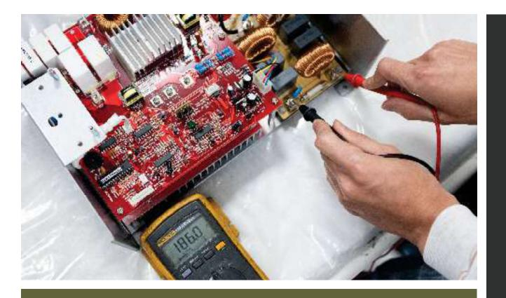
Inspect the fuse and power supply parts
