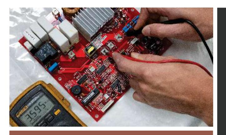
• Measuring G&C and you should get a very high resistance such as  $3.59M\Omega$  if it is under normal condition.
