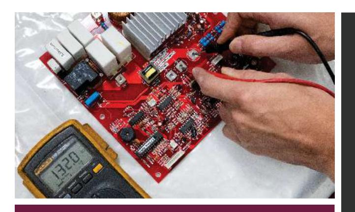
• Measuring E&C and you should get  $130K\Omega$  if it is under normal condition.
