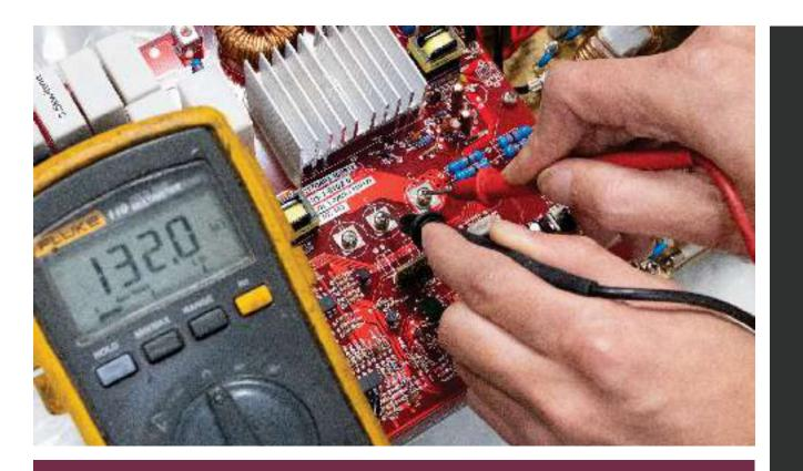
Measuring E&C and you should get something around 130KΩ if it is under normal condition. If not, it means either the mainboard or the IGBT module has failed.
