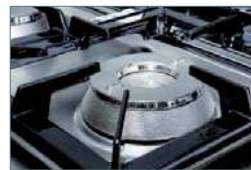
Open burners with 1-crown burner of 4.5 kW or 2-crown burners of 8 kW with possible combinations depending of number of burners of each model. Robust crowns with high-efficiency burners and provided with a flame safety device. Pilot ignition covered to avoid the breakage.
